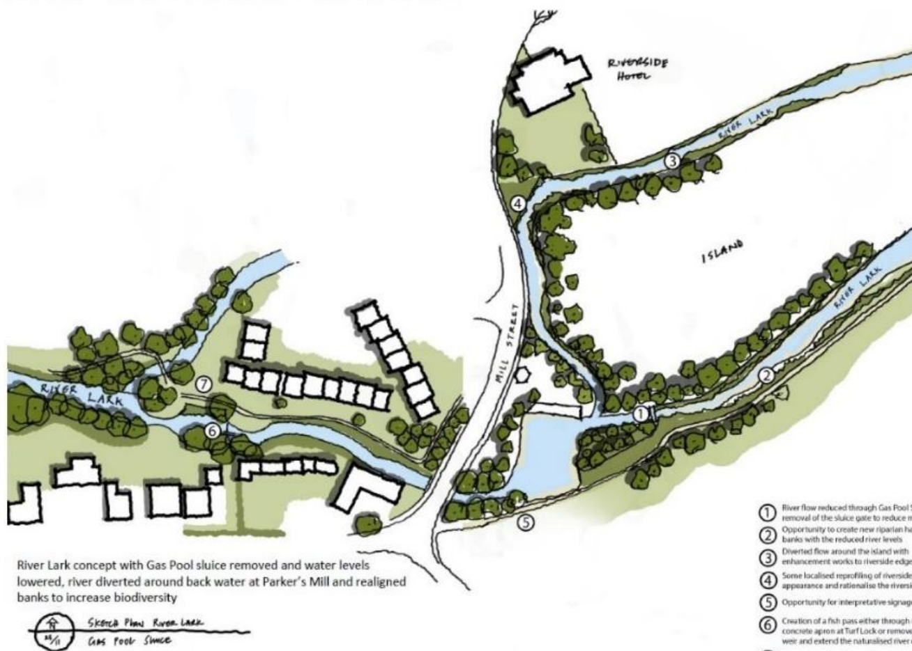
Fig 13. Option 1, Gas Pool sluice filled in and weir removed back channel created and both channels lowered to hard bed.
